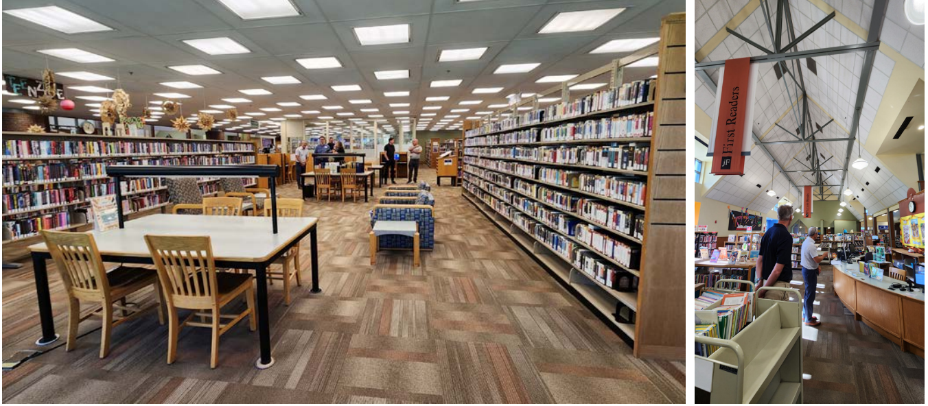
Large stacks obstruct sightlines to gathering and seating spaces; cathedral ceiling amplifies sound from children's area
